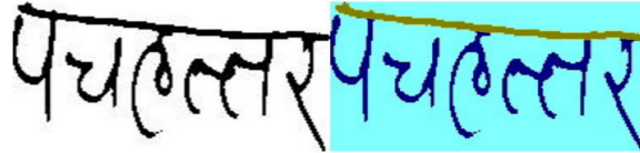
Fig.1 Segmentation of a handwritten Devanagari word into pre-defined classes by using pixel-labelling. Background, Characters, and Shirorekha represented with turquoise blue, Persian blue and citron brown, respectively.
