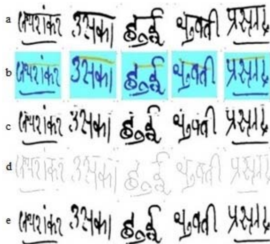
Fig.10 An illustration of segmentation achieved on script-dB (a) original images (b) ground truth (c) segmentation achieved with Seg1 (d) segmentation achieved with Seg2 (e) Segmentation achieved with ShirorekhaNet .
